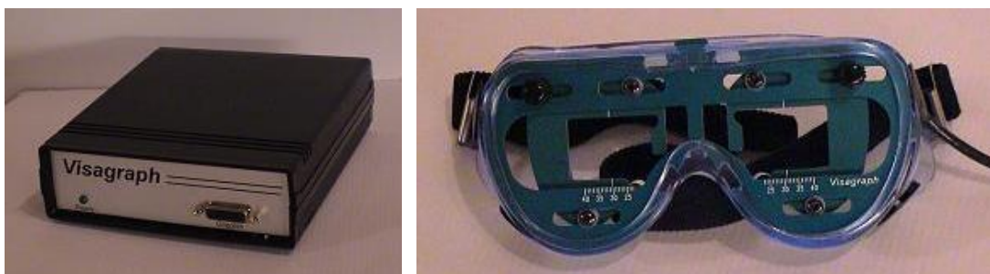
Figure 1: Visagraph™ III components: measuring unit, which is connected to a computer with the analysis software (left) and eye tracking goggles (right) [38]
